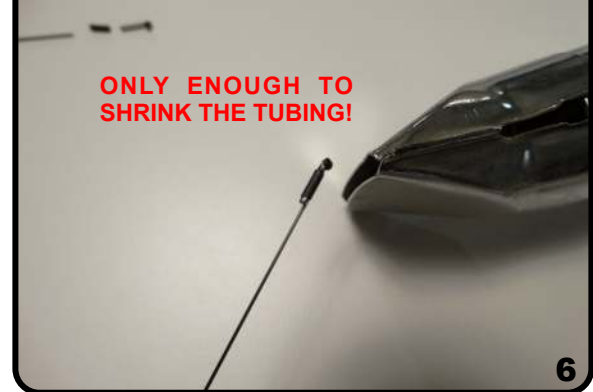
Attach link in saddle area, slide tubing on and heat
