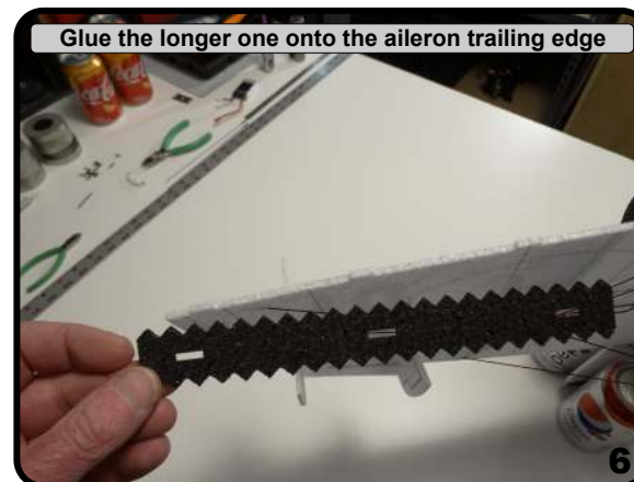
... and square to the control surface
