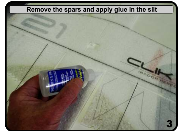
Constrain flat and let sit for a bit
