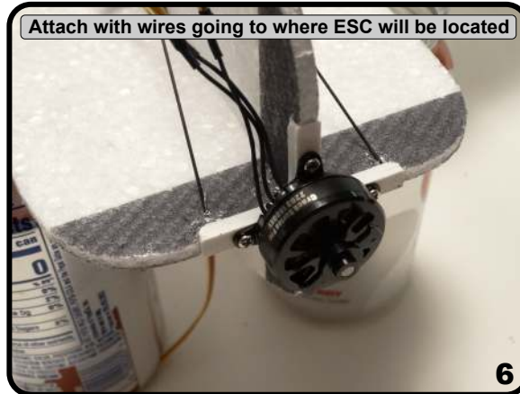
Mount ESC and Receiver approx. where shown
