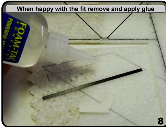
Make sure the horn hole is over the hinge center
