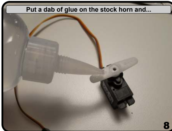
...attach the Diff Horn - Keeping center holes aligned
