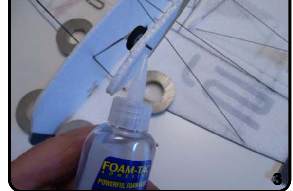
Make sure the wheel can spin and add a dab of glue
