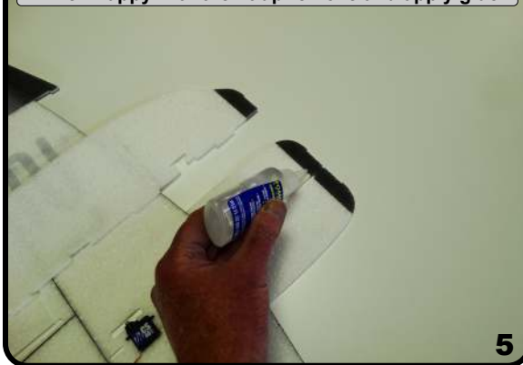
When happy with the fit up remove and apply glue
