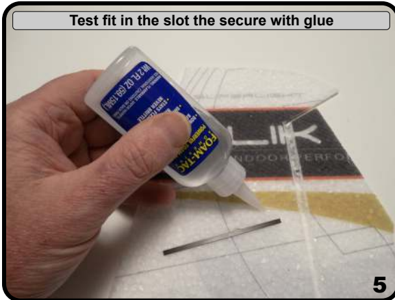
Put some glue on the horn and intall as shown
