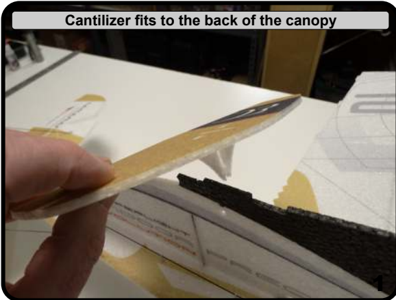
When happy with the fit up, glue mating surfaces
