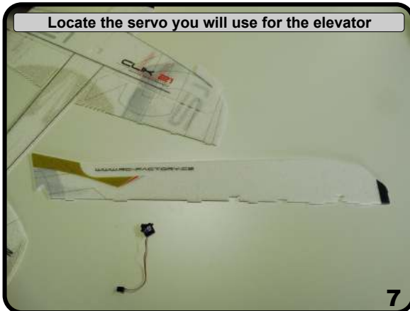
It will install into the cutout in the horizontal section
