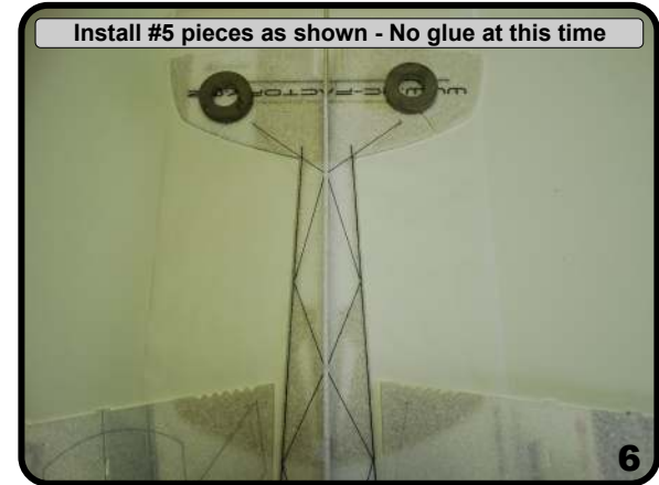
Make sure the fuselage is nice and straight
