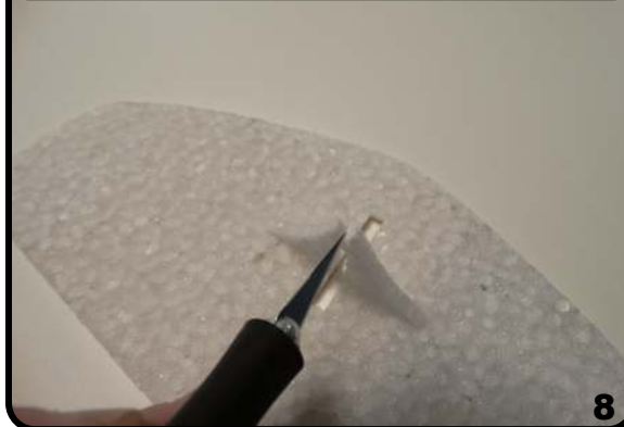
With a sharp hobby knife slit the top tab
