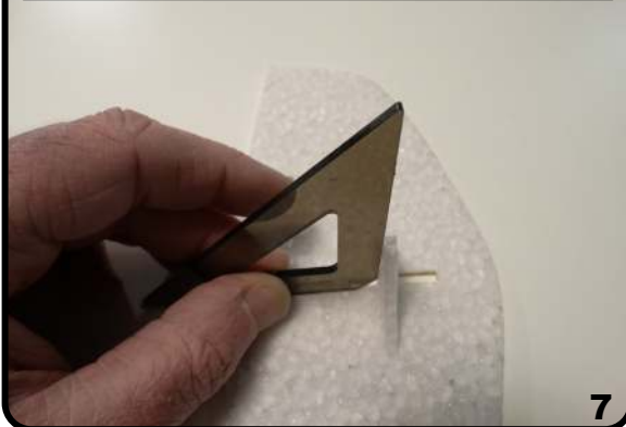
Bring the pieces together and check for square
