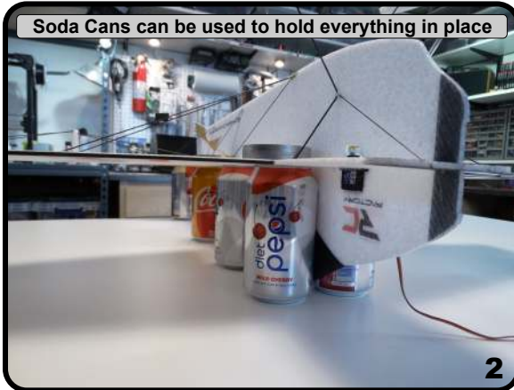
Test fit in the slot the secure with glue
