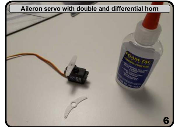
...attach the Diff Horn - Keeping center holes aligned
