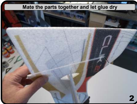
Should go all the way top to bottom and be flush
