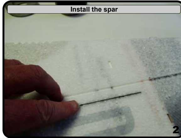
... make sure it is flush, and let sit for a bit
