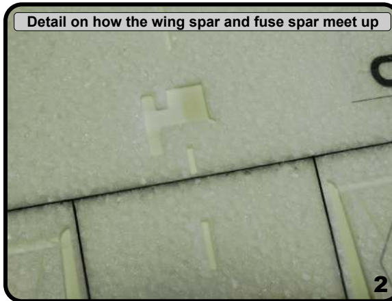
While the glue is wet - make sure fuse is straight
