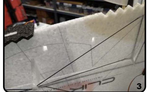
Clear/Cut the holes shown in the wing
