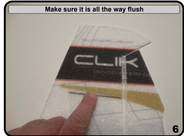
Test fit the rudder
