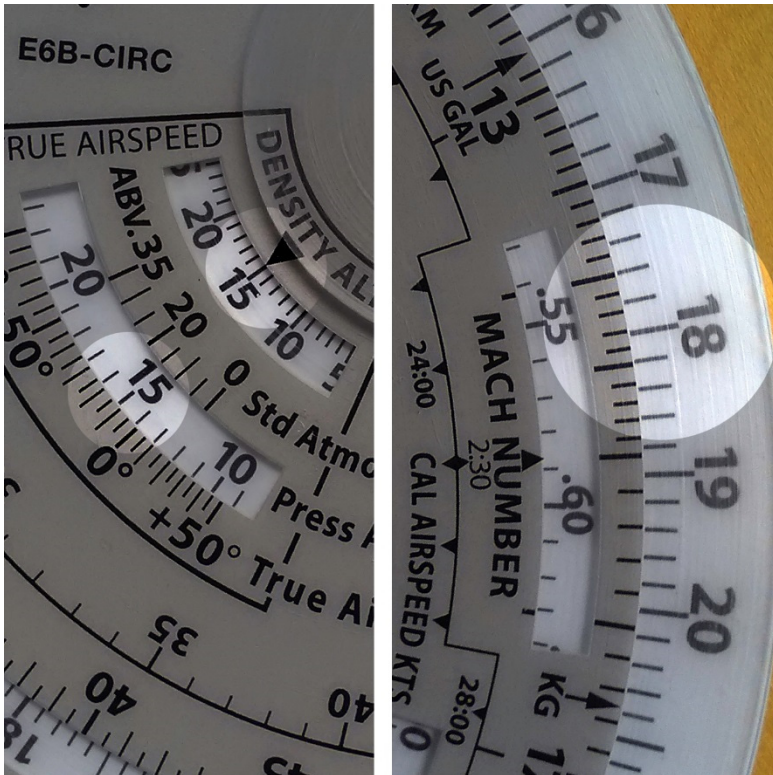
Figure 14. Align outside air temperature opposite the pressure altitude then read density altitude over the arrow.
