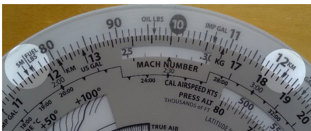
Figure 5. Set the SM value under the SM arrow and read the corresponding KM value under the KM arrow.
