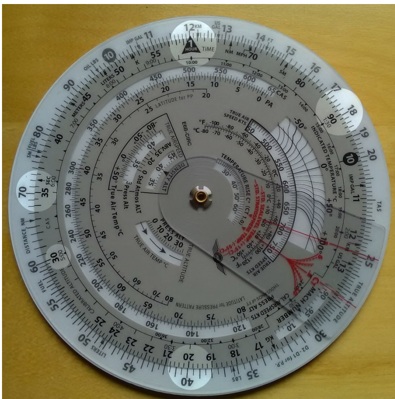
Figure 3. Line up the 1 triangle (the rate arrow) with the number 12 on the outer disk (scale).
