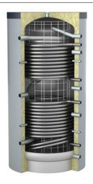
With this OEG hygienic storage tank, the highest demands on the hygiene of drinking water and energy efficiency are fulfilled. The structure of this tank is fundamentally different from usual, large-volume service water tanks. A built-in corrugated stainless steel pipe separates the drinking water from the heating water and - at the same time - serves as a powerful heat exchanger. Thus, the advantages of a buffer tank are combined with those of a hot water heater.
