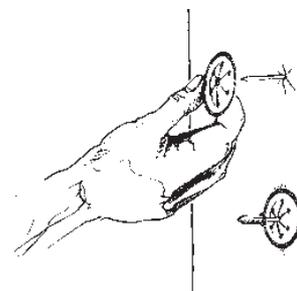
Insulation can be impaled immediately and firmly locked with locking washers, but maximum strength of adherence is achieved after 24 hours. If necessary, cover the pin with protective cap.
