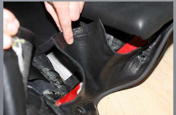
7. Close leather flap and fold forward, fasten screws if necessary
