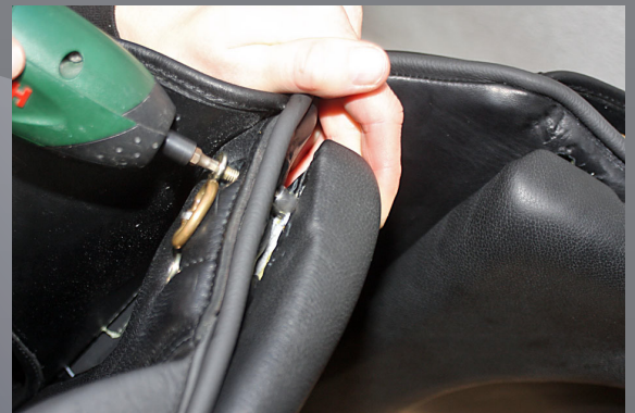
8. Fasten screw(s) from outside
