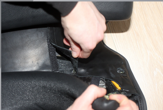
3. Remove small screws if necessary, open leather flap and fold forward
