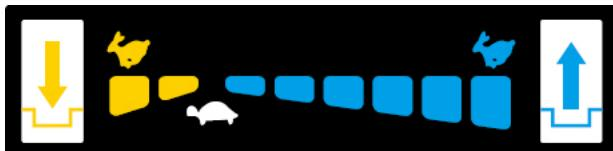
The speed shift lever has 8 positions: 6 forward speeds and 2 reverse. To change speeds, move the speed shift lever to the desired position. The lever locks in a notch at each speed selection.
