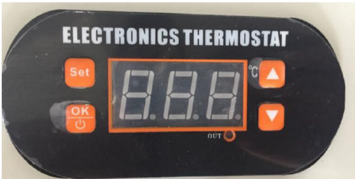
Press "OK" to turn on the temperature controller indicating the real-time temperature.
