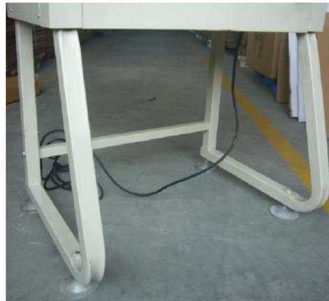
1. Lay down cabinet; connect two support legs (23) with cabinet using four M12 Screws and Flat Washers.
