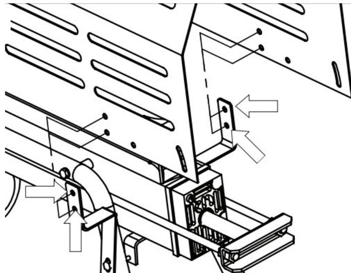
Connect the side cover with the machine with 2pcs of outside hex bolts M8x16, gaskets  $\varnothing 8$  and lock nuts M8, and with 4pcs of outside hex bolts M6x12.
