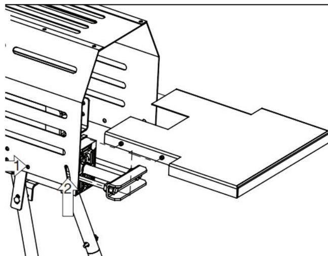
Connect the log catcher with the cover with 2pcs of outside hex bolts M6x12, gaskets  $\varnothing 6$ , lock nuts M6 and 2pcs knobs and gaskets  $\varnothing 6$ .
