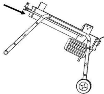
Periodically check oil level to ensure it is between 2 grooves around the Dipstick. Upon lower oil level, oil refilling is required.
