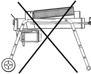
Break log in the direction of its growing grain. Do not place log across the log splitter for splitting. It may be dangerous and may seriously damage the machine. Do not attempt to split two pieces of logs at the same time. One of them may fly up and hit you.
