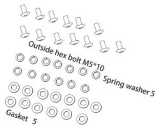
Connect the whole cover with 13pcs of outside hex bolts M5x10, spring washers  $\varnothing 5$  and gaskets  $\varnothing 5$ .
