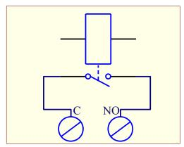
Schematic outlines of how the relay outputs are implemented internally
