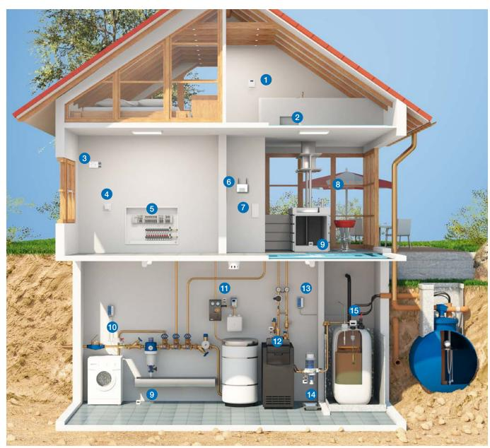
A fully featured smart building system on the basis of EnOcean wireless technology networks all light, heating and air conditioning control systems via a central gateway. The gateway processes sensor and consumption data, triggers control action and initiates other measures, and transmits the information to mobile devices such as smartphones, tablets, etc., via WLAN, Internet or GSM. Products from other members of the EnOcean® Alliance for controlling household appliances can also be integrated.
