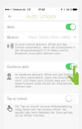
If the geofence setting is active, the lock will open automatically only if the smartphone was at least 500 meters away from the lock. As long as you are within a radius of 500 meters around home, it does not open automatically. For this feature, you should enable Wi-Fi on your smartphone.
