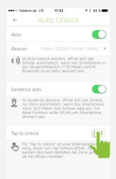
In "Tap to unlock" a declaration of will is necessary before the lock opens. When entering the auto-unlock zone you will be asked if the lock should be opened. You can confirm this interactive notification with "Open".
