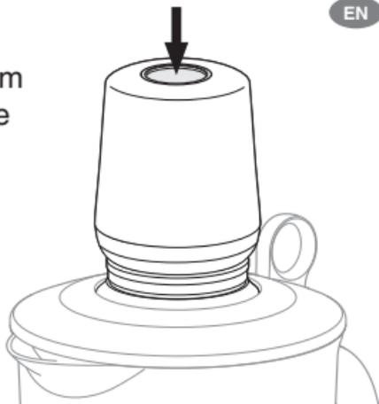
7. Press the Vacuum Valve to release vacuum pressure from the blender jug.
