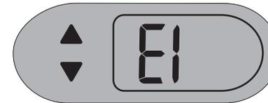
The mixer is equipped with an electric protection cut-off and will automatically stop operating if the motor is stalled or overloaded. This is normally due to excessive quantity in the mixing bowl.
