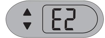
The mixer is equipped with a self-resetting safety device which safeguards against overheating the motor with excessive loads. If overheating occurs, the mixer will automatically activate the overheating protection device and the motor will switch itself off. If this error occurs, turn the speed control dial to the 'OFF' position, switch the appliance off at the power outlet and unplug the cord. Wait at least 15 minutes before restarting the mixer.
