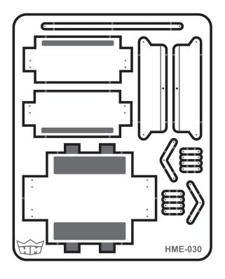
Cut parts from sheet carefully with sharp knife.
