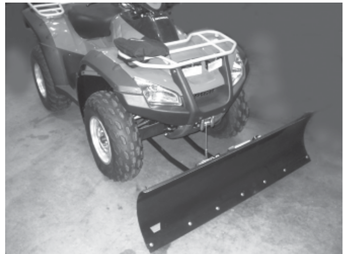
Figure 8 Completed Winch and Plow Assembly
